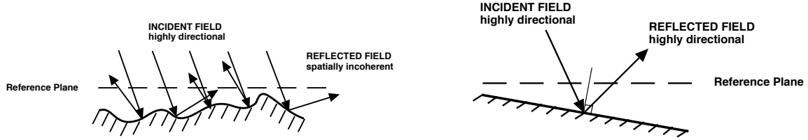
Figure 2. Left figure: rough surfaces give diffuse reflections. Right figure: smooth surfaces give specular reflections.
