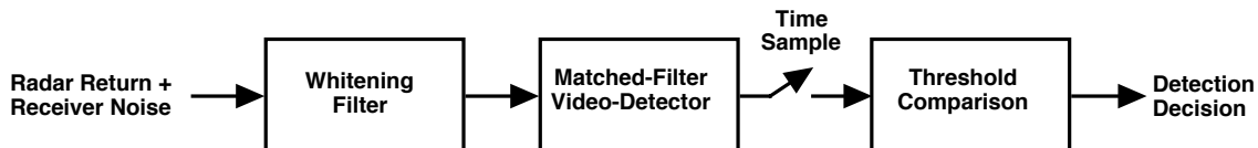
Figure 5. Optimum Neyman-Pearson receiver for a specular target embedded in diffuse clutter plus receiver noise.
